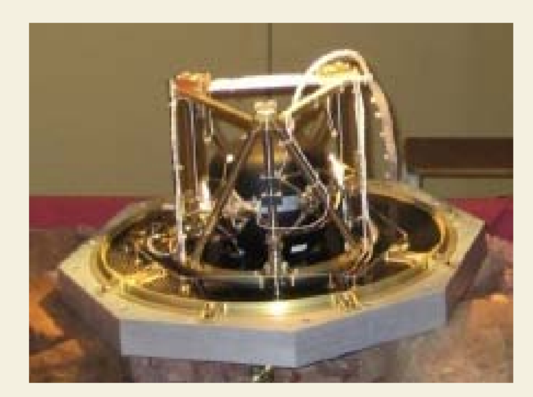
Fig. 4: Instrumented SPHERE on a ExoMars Leveling (LVL) system prototype (courtesy MPS)
